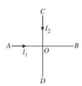
$$B = (B_1^2 + B_2^2)^{1/2} = \left[ \left( \frac{\mu_0}{4\pi} \frac{2I_1}{d} \right)^2 + \left( \frac{\mu_0}{4\pi} \frac{2I_2}{d} \right)^2 \right]^{1/2}$$
