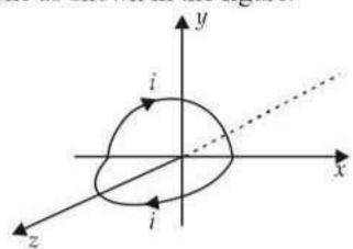
Magnetic field at the centre due to semicircular loop
