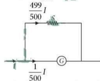
As shunt and galvanometer are in parallel
